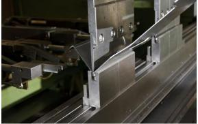
A Hydraulic sheet metal bending machine is used for bending the sheets into required shape and size. The metal joints are spot welded and then transported for JAGUAR furniture Mysore for power coating and then transported to mnay retail shops and residences.
