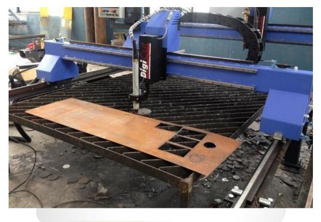
A Hypertherm made CNC plasma cutter with digicut nozzle is used to cut the sheets into a proper size and then further process.
